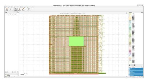
Figure 21. Display of user project wrapper in klayout
